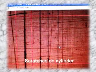
After rotations shoe is worn away, sometimes it makes scratches on your cylinder as upper-right photo.
